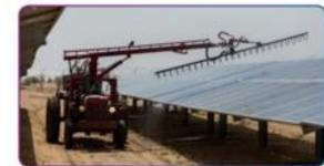
Innovation in Module Cleaning System (Semi - Automatic)
